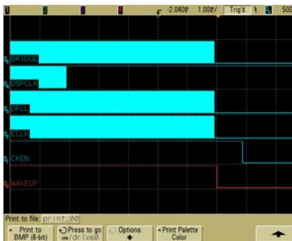
Figure 4.0 Locosto signals – ACTIVE to DEEP SLEEP sequence
